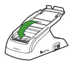
❖ If the device prints blank receipts, insert the paper roll the other way around.
